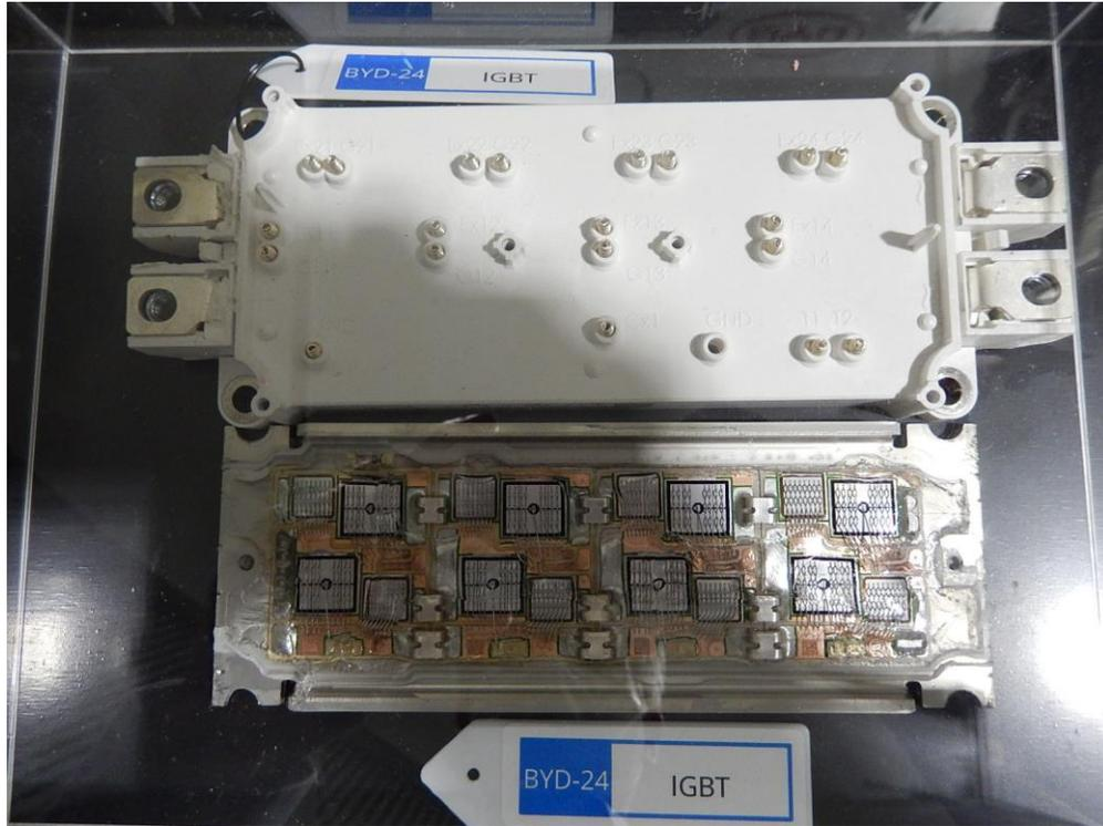
IGBT(Insulated Gate Bipolar Transistor)とは
